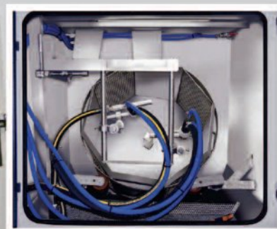
The Aquablast® Tumbler machine with a 2-stage optional hot and cold rinse. This machine batch processes small parts which are gently tumbled in the drum while being simultaneously blasted.
